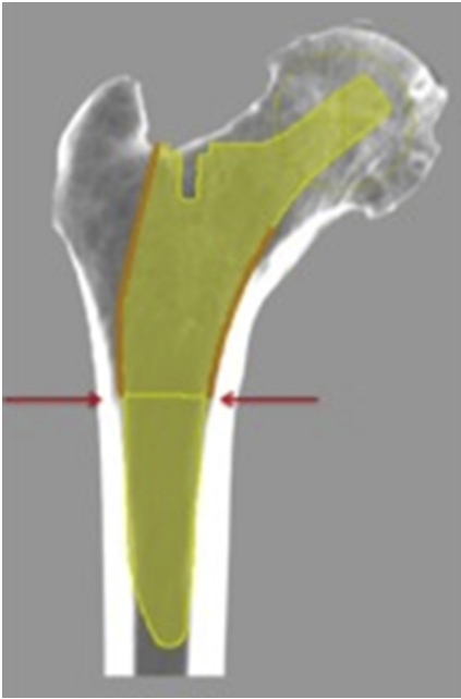
Fig. 7. Two-point wedge fit design. The implant is designed to contact the medial and lateral cortices at the metaphyseal-diaphyseal junction.
