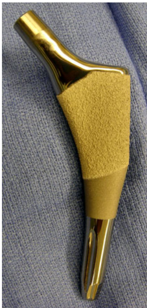
Fig. 1 The off-the-shelf implant consisted of a polished titanium alloy with a hydroxyapatite coating on a titanium plasma spray in the proximal 1/3 of the stem.
